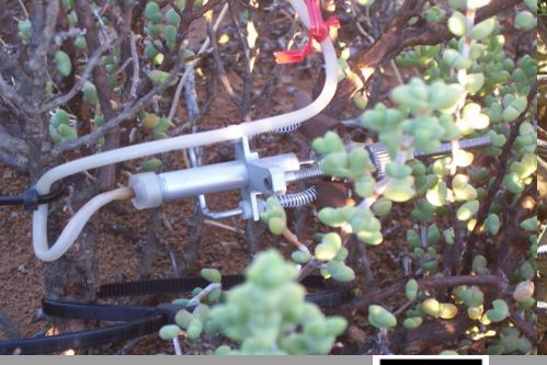
Stem microvariation sensors interfaced with logging unit
