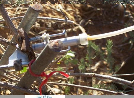
Stem microvariation sensors interfaced with logging unit
