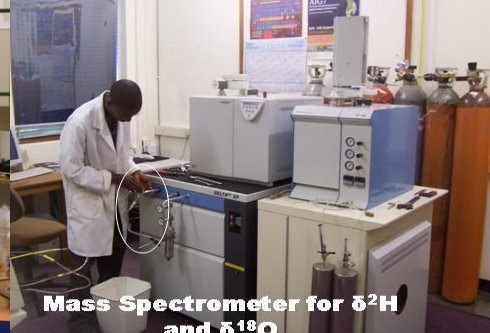
Preparation of samples for \delta^{18}\text{O} & \delta^2\text{H} mass spectrometry
