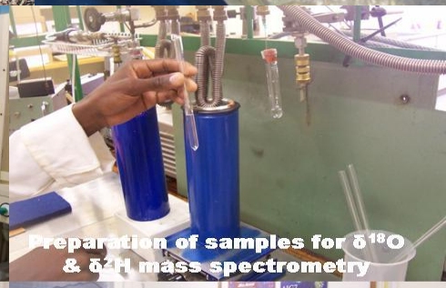
Cryogenic extraction of xylem water
